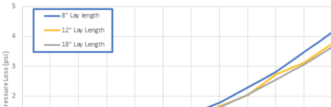
1.5" Swing Joint Pressure Loss (0-60 gpm)
